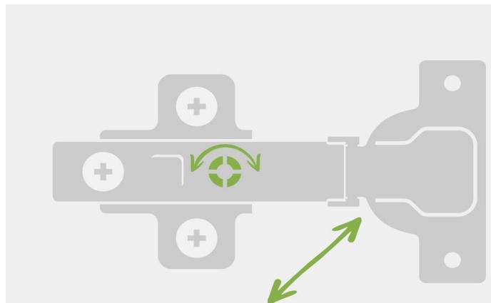
The front screw can be used to adjust the width of the door.
