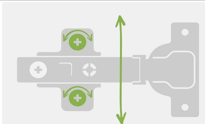
Loosen the two screws of the mounting plates, adjust the height of the door, tighten the screws again.
