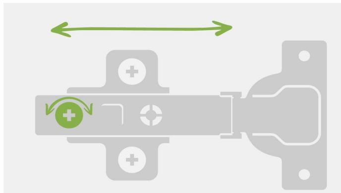
The rear screw can be used to regulate the distance (gap) between the door and the furniture.
